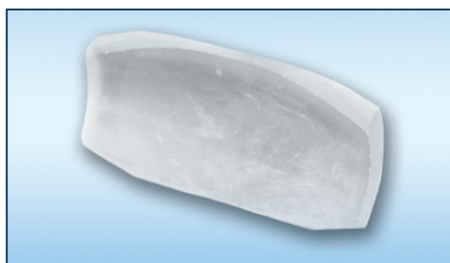
Toroidal monochromator. R1=150 , R2=75 , LiF(200), 2d=0.403 nm
