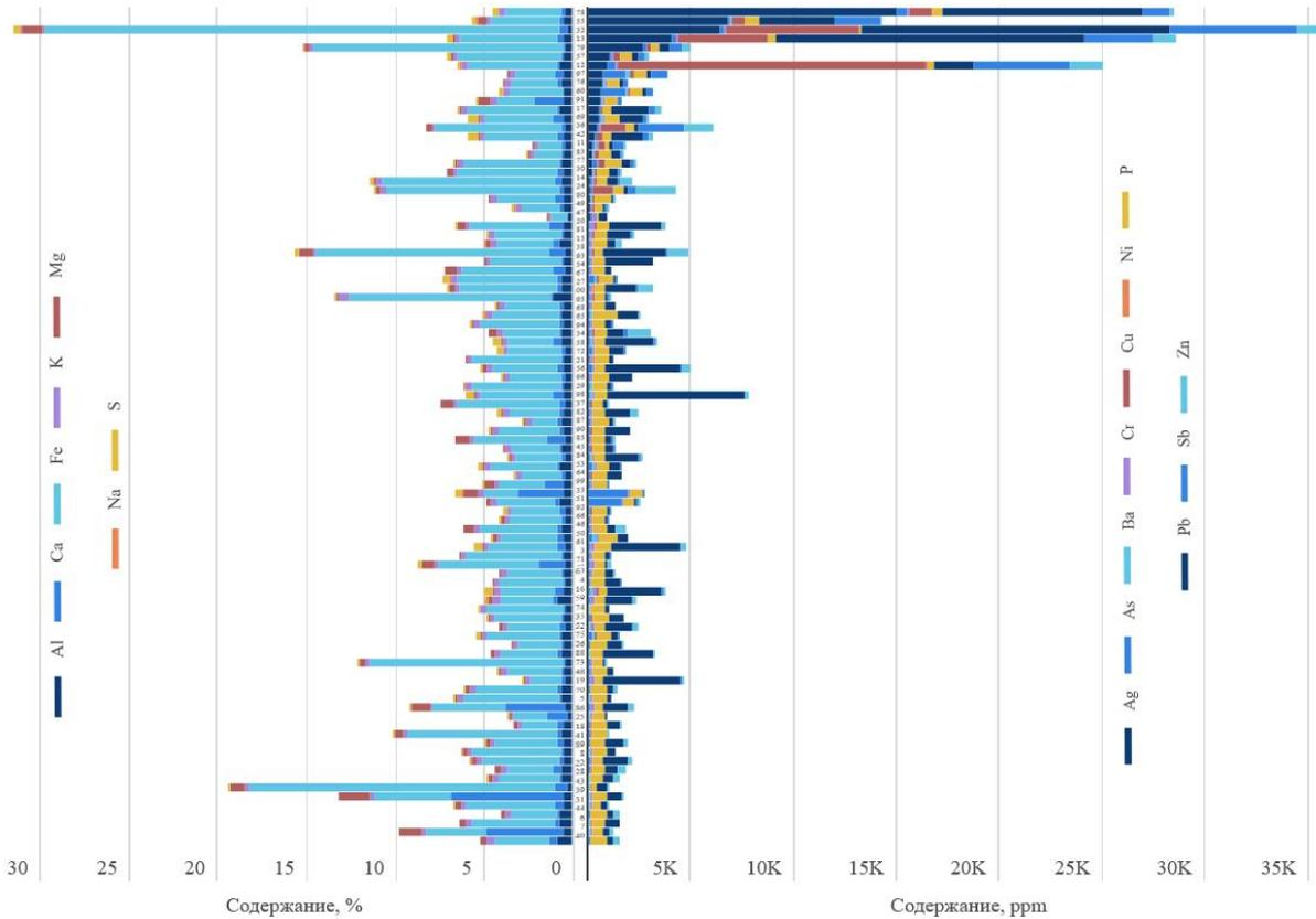
Results of quantitative composition of chemical elements in silver-bearing ore samples obtained by inductively coupled plasma AES method
